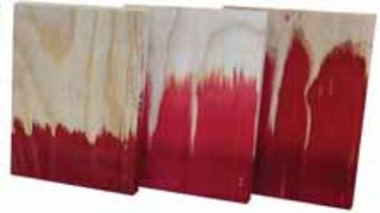
When exposed to similar conditions, plywood panels absorb more water than AdvanTech floor panels, which can lead to swelling and delamination. AdvanTech floor panels resist moisture penetration, preventing moisture-related damage.
